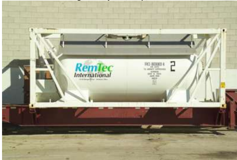
Figure 36: One of RemTec's multimodal shipping tanks, used for shipping refrigerant by rail, ship, or truck
