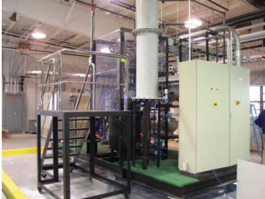
Figure 35: A PLASCON® plasma arc destruction unit
