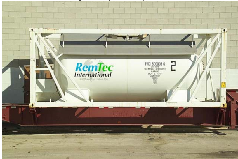
Figure 17: One of RemTec’s multimodal shipping tanks, used for shipping refrigerant by rail, ship, or truck
