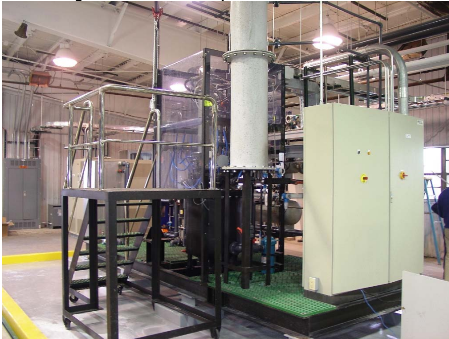
Figure 16: A PLASCON® plasma arc destruction unit
