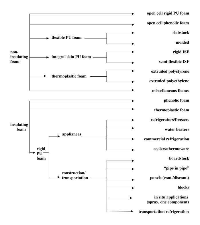
The most prevalent use of **open cell rigid PUR foam** is for packaging applications ("pour in place" foam), mostly when small lots are involves, such as in the return of repaired items. Another application is "back-foaming" of crash panels, such as automotive dashboards.
