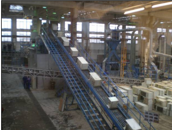
Exhibit III-3: The Praktik demanufacturing facility, with two segments of the disassembly line shown
