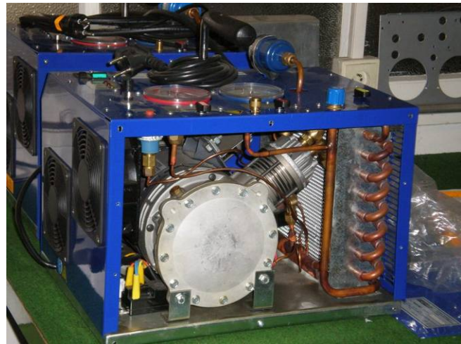
Exhibit III-4: The inner workings of a recovery unit manufactured by Ekotez
