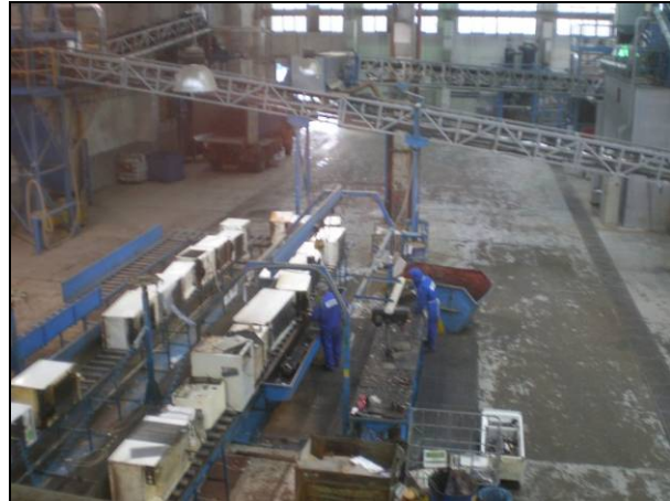
Exhibit III-3: The Praktik demanufacturing facility, with two segments of the disassembly line shown
