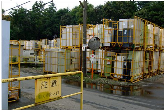
Exhibit V-3. Kanto Eco Recycle (KAREC) Home Appliance Recycling Plant. Domestic appliances are stored at Kanto Eco Recycle prior to processing. Appliances are transported and stored in specially-designed crates to maximize efficiency. Located on the outskirts of Tokyo, this facility recycles all four types of household appliances.
