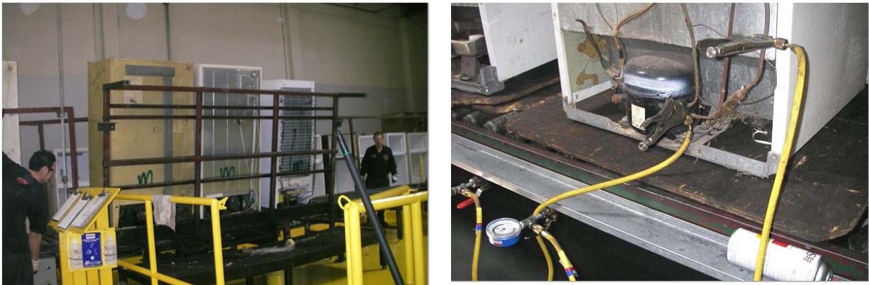
Exhibit VII-2: Refrigerators at ARCA, Inc. (Appliance Recycling Centers of America) awaiting processing (left) and being drained of refrigerant (right).
