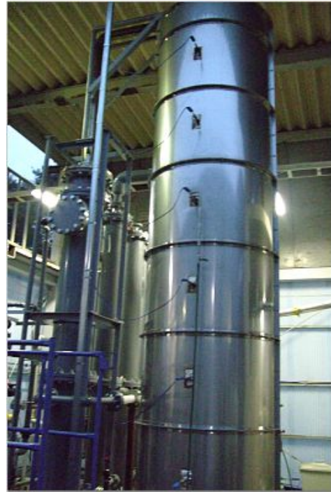
Exhibit V-9. Kankyo Soken's Refrigerant Reclamation Technology and Catalytic Fluorocarbon Decomposition Plant
