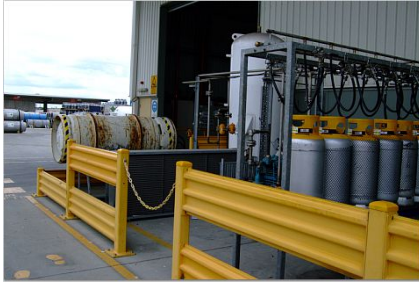
Exhibit I-9. Refrigerant Decanting into Bulk Storage at A-Gas, Prior to Transport to RRA for Destruction
