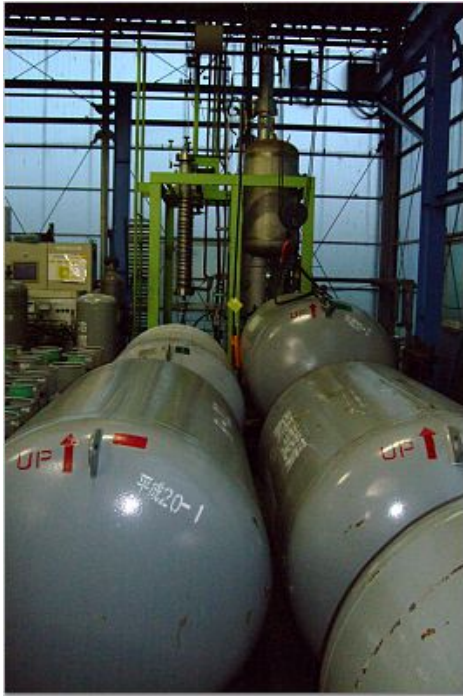
Exhibit V-9. Kankyo Soken's Refrigerant Reclamation Technology and Catalytic Fluorocarbon Decomposition Plant
