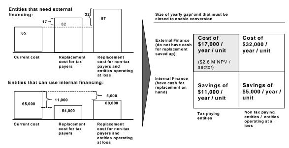
Assumptions: 300 TR chiller, .56 kW / TR power consumption (replacement), .7 kW / TR power consumption (baseline), 9 hours/ day, interest rate 20%, aggregate upfront taxes waived for chiller equipment, down payment 0%, loan term 10 years, chiller price \$150,000, installation \$30,000.
