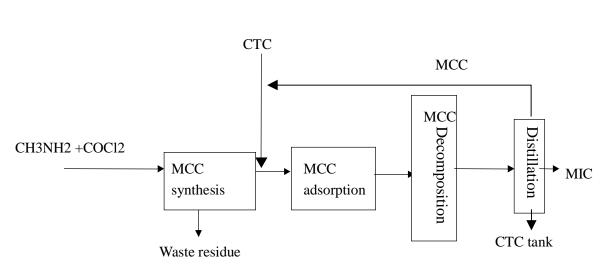
The flow sheet for the production of MIC intermediate is as follows.
