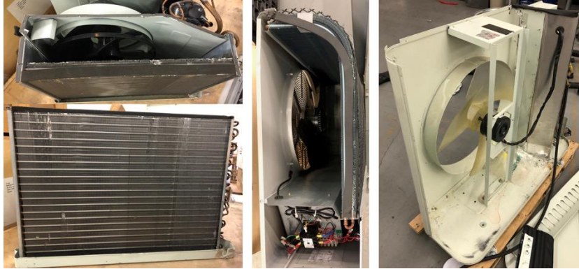
FIGURE 10. CONDENSER FORMS: UNIT 1 (LEFT), UNIT 10 (CENTER), UNIT 6 CABINET (RIGHT).
