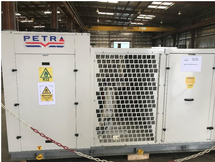
Figure 7: R-32 Prototype with Markings
