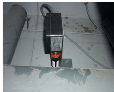
Figure 5.12: Additional sensor installations in the HC-290 recharging chamber.
