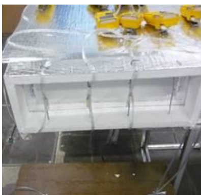
Figure 61: Sampling matrix for horizontal main duct
