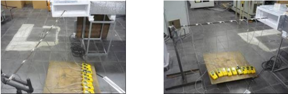
Figure 69: Arrangement of sampling points to determine extent of flammable mixture exhausted from the single duct outlet
