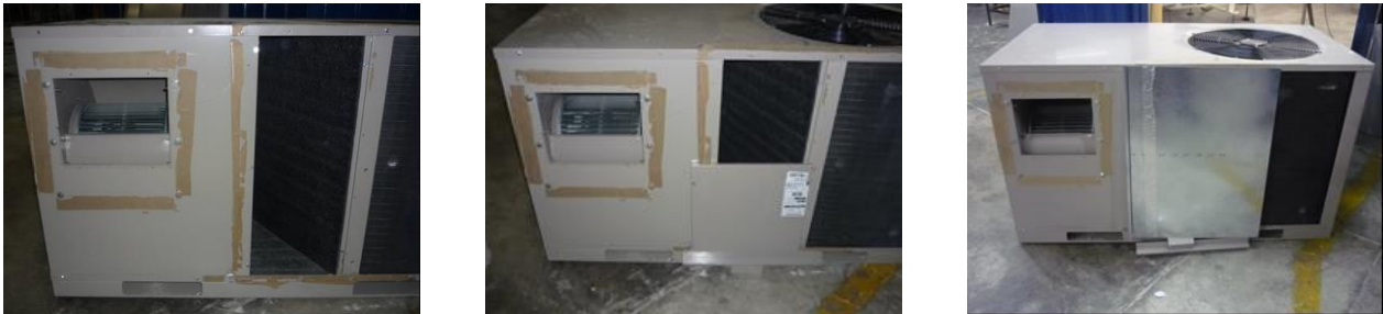
Figure 75: Rooftop unit return air inlet fully open, half blocked and fully blocked
