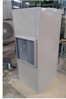
Figure 105: Redesign of AHU with internal plenum chamber
