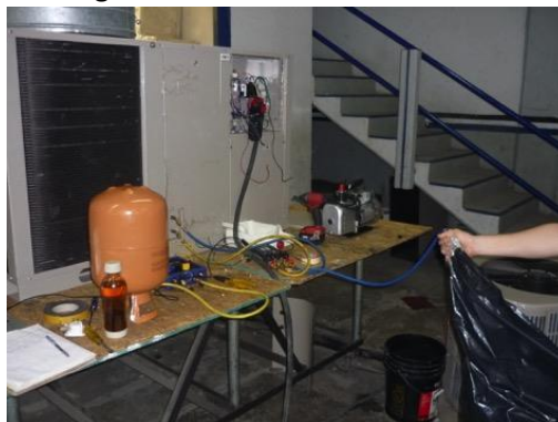
Figure 10: Photograph of test arrangement, where refrigerant hose is connected from leak position and fed into collection bag for measuring once test is finished
