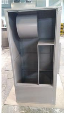
Figure 105: Redesign of AHU with internal plenum chamber
