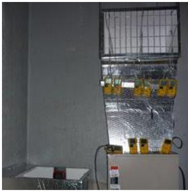
Figure 54: Sampling matrix for main duct
