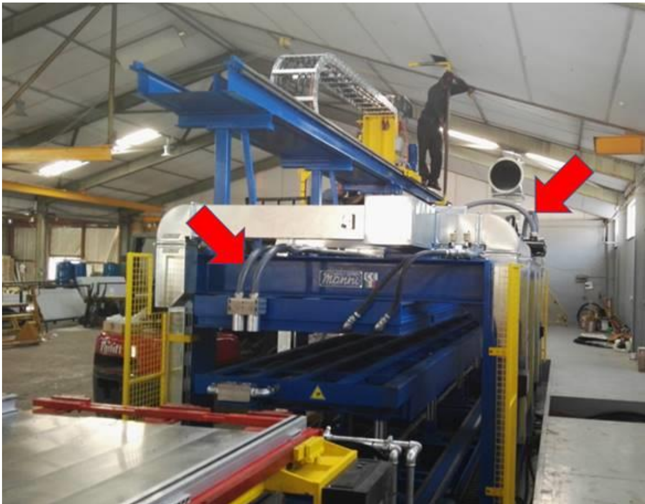
Manni press 2+2 equipped with vacuum device Release of vapors with Pentane as blowing agent
