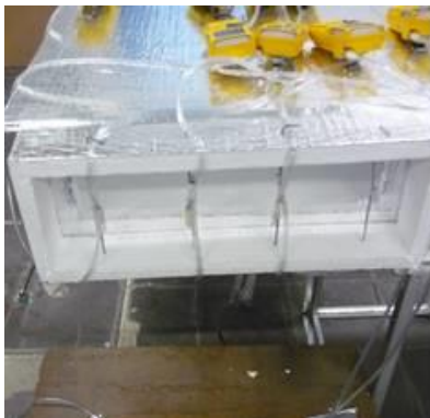
Figure 61: Sampling matrix for horizontal main duct
