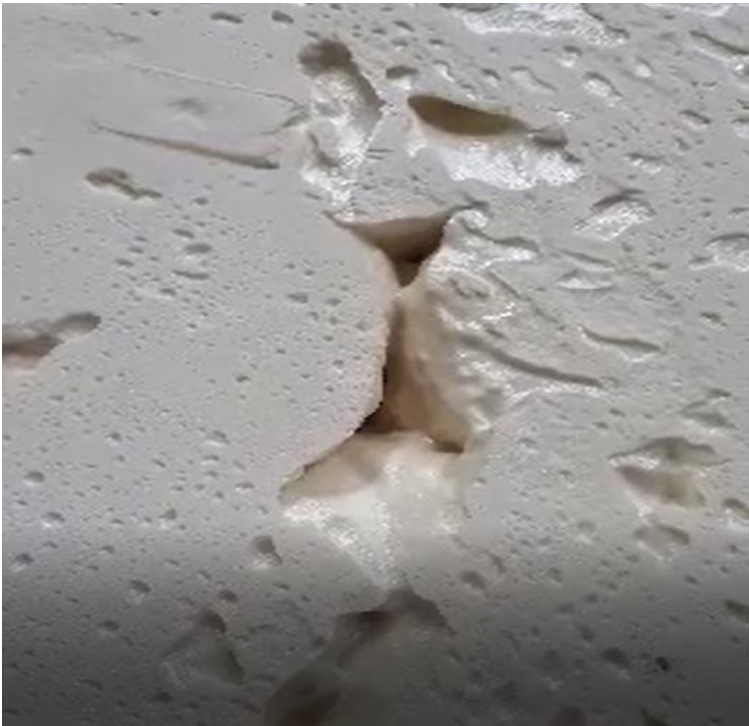
Air voids trapped inside the foam
