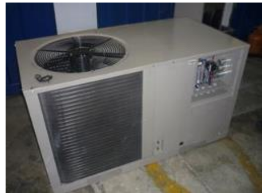
Figure 38: Photographs of models used for testing; ducted split (left and centre) and rooftop unit (right)
