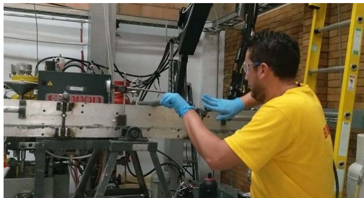
Figure 5. Measurement of foam expansion at Brett mould
