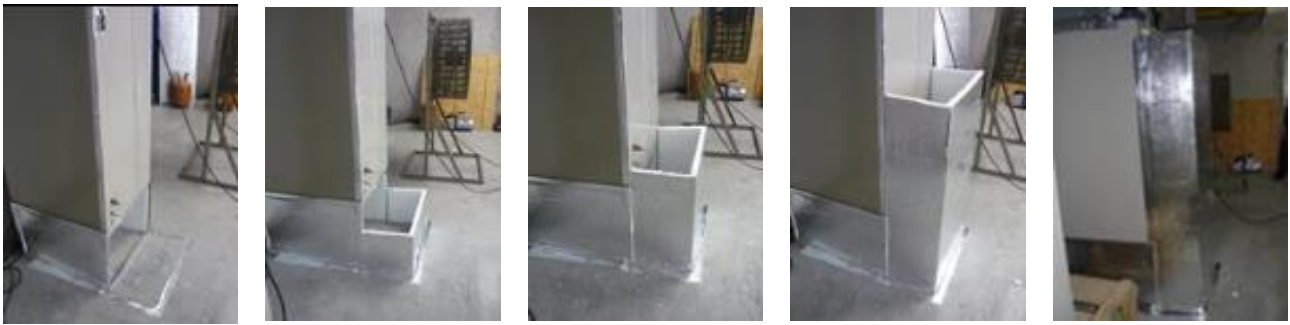
Figure 101: Different elevations of outlet plenum; from left to right – 0.0 m, 0.25 m, 0.50 m, 1.0 m and 1.5 m
