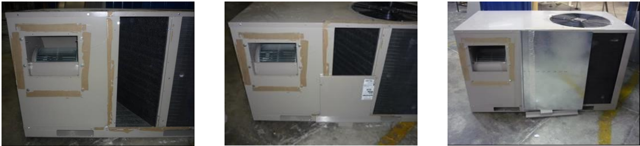
Figure 75: Rooftop unit return air inlet fully open, half blocked and fully blocked
