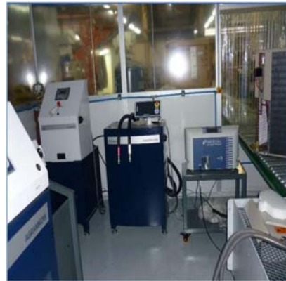
Figure 4.19: Storage compartment of R290 refrigerant gas (capacity: 4 cylinders, 5.5 kg each); charge and leak test equipment.
