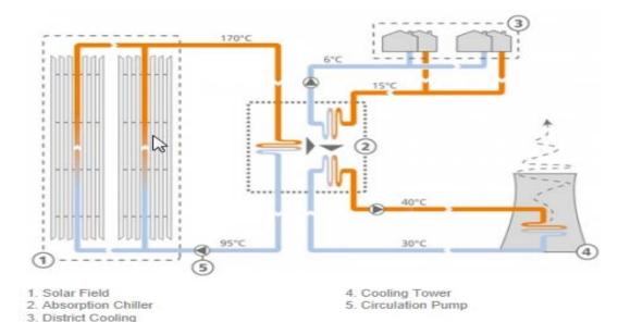
The increasing requirement for cooling can be produced most economically by district cooling systems with a correspondingly large solar field. The cooling energy is carried to the respective consumers in transmission line networks. District cooling systems are becoming the popular choice in high temperature locations including the Middle East. Novatec Solar's system provides the sustainable solution to the district cooling and refrigeration demands of these regions.
