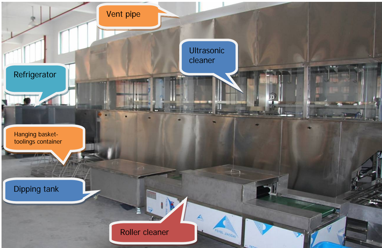
Pic4: the needle-making clamp cleaning line
