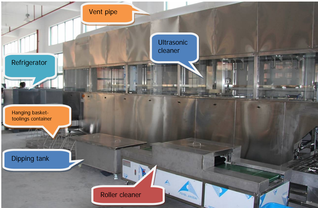
Pic4: the needle-making clamp cleaning line
