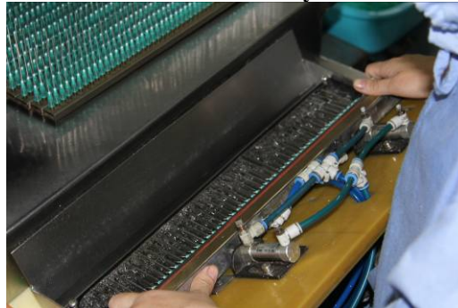
Pic10: Needles Silicification by hand
