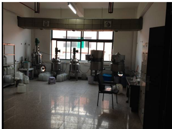
Pic25: Special room for silicification fluid management with vent pipe and fire pipe
