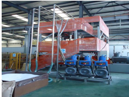
Feeder and gravimetric dosing system for PS resin
