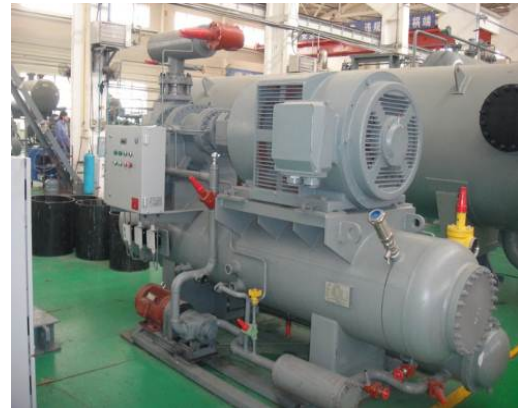
Fig 11. L20R compressor and system
