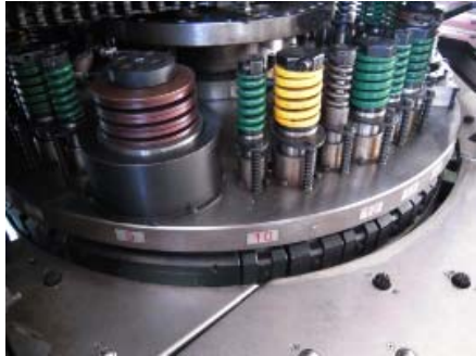
Die for end-plate hole-punching
