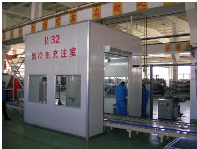
R32 charging room
