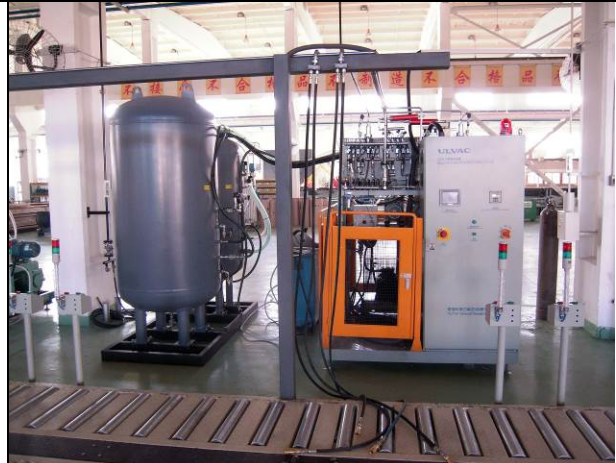
Helium refrigerant recovery machine
