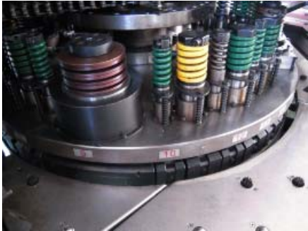
Die for end-plate hole-punching
