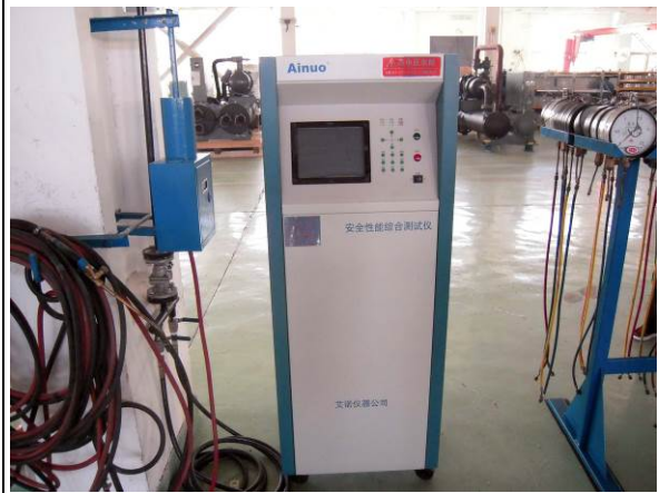
Testing equipment for electronic safety performance
