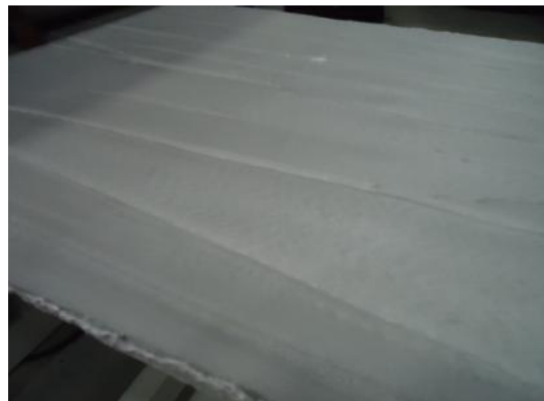
Picture 6- The photograp of the product which the gas blend is 80/20 HFO1234ze/DME %1 Nucleating agent.
