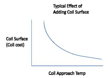
The approximate range of coil approach temperatures for evaporator and condenser coils is between 20 °F (1 row smooth bore tube coil) to 10 °F (4 row IE tube). 10°F is nearly a practical limit.
