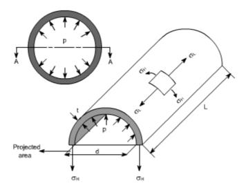
If the ratio of the thickness to the internal diameter is less than about 1/10 then it can be considered as thin-walled cylinder. It is assumed that the hoop and longitudinal stresses are constant across the thickness. It may also be assumed that the radial stress is small and can be neglected. Under thin-wall assumption, hoop stress can be calculated using the following equation:
