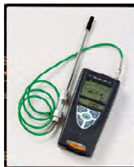
METHYLAL EMISSIONS DETECTOR 0-2,000 ppm
