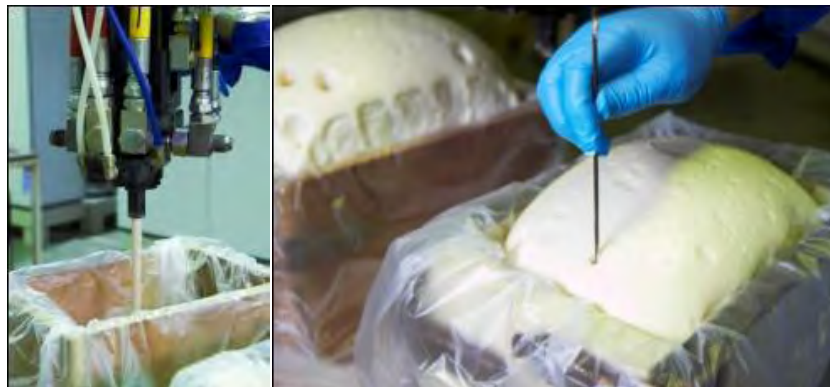
Picture 5,6: Extraction from brett mold, injection in jumbo mold and extraction of produced foam
