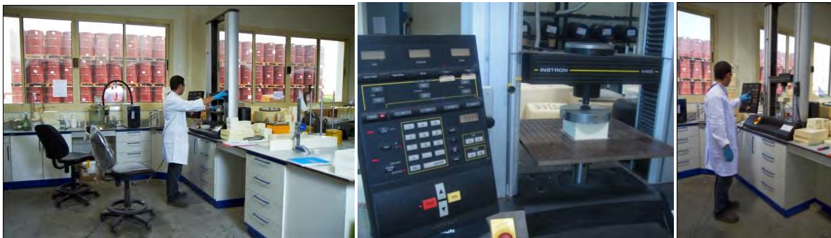
Picture 8,9: compressive and tensile strength testing with dynamometer
